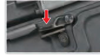
Release the dummy bolt by pressing the bolt release button before closing the eject port cover.
